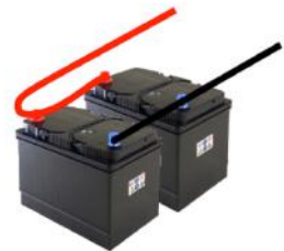
Figure 4: Recommended wiring for connecting batteries in parallel.
