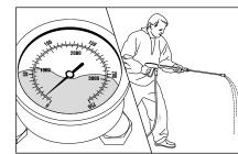
The stainless steel pressure gauge shows low pressure despite fully turned up pressure regulation. The water from the lance comes in squirts. The high-pressure hose vibrates.
