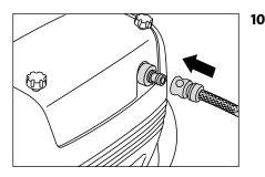
10. Connect water hose to water inlet (minimum requirements; 5 m hose length, cross-section ¾", 10 bar). The high pressure cleaner may be connected to a water mains (1-10 bar pre-pressure) with either cold or hot water (up to 60 °C). The large quadro series provides the opportunity of sucking in water out of a container (see direct suction).
