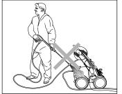
Never direct the high-pressure jet at the highpressure cleaner itself! The high-pressure cleaner may not be placed within reach of the highpressure jet spray mist!
