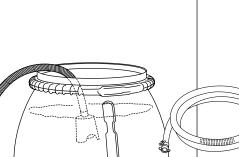
Suction hose with suction filter With return valve Hose length 3 m
