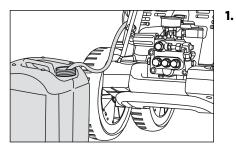
Place chemicals filter into container with additives
