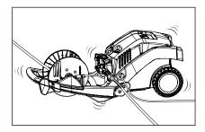
Having closed the safety trigger gun, the high pressure cleaner must shut down. Failure to shut down may be caused by leakage in the high pressure pump, the switch, the high pressure hose, the safety trigger gun or the lance.
