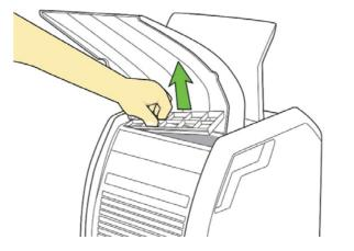
To attach the focus enhancer, first remove the grill that comes with the unit. Ensuring that the filter sponge is still in place, attach the focus enhancer in the place of the existing grille.It should snap into place. If it does not, ensure it is inserted with the correct orientation. The nozzle should be facing inward as shown in the diagrams.
