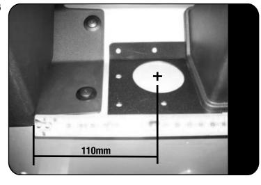
Looking inside the vehicle, place the center of the Inlet Cover Plate (Item 4) 110mm from the speaker box.
