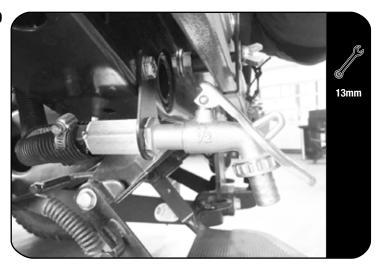
Run the tap assembly toward the rear left of the bumper. Secure the locking tap to the bumper using a M8 x 80 Hex Bolt, two M8 Flat Washers, and a M8 Nyloc Nut (Item 10, 11 & 16).
