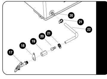
Wind thread tape around the thread Barbed fittings (Item 20). Screw one Barbed Fitting into the water tank outlet.
