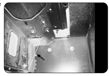
There is a fender support bracket that needs to be modified. Using your grinder cut the gusset section of the bracket as close to the body as possible Using a hammer, form the remaining part of the bracket so that in is flush with the body of the vehicle.
