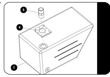
Lift the Water Tank (Item 1) into position under the fender.
