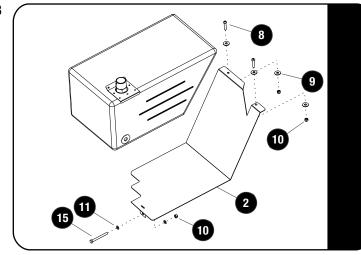
Place the Tank Protection Plate (Item 2) underneath the tank.
