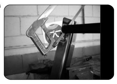
The safety support bracket must be modified. Clamp the 'flat' portion in a vice. Using your hack saw, cut the tube off as close to the plate as possible.
