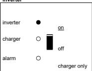
The inverter is switched on and supplies power to the load. Battery operation.
