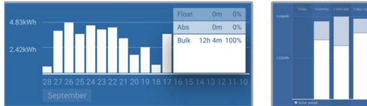
System spending all its time in bulk with breakdown of charge stages - System in bulk and absorption
