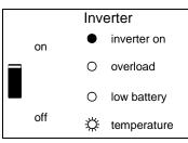
The internal temperature is reaching a critical level.
