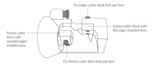
Check cutter block bolts for tightness before each use. Use protective gloves when handling cutter blocks as edges are very sharp.
