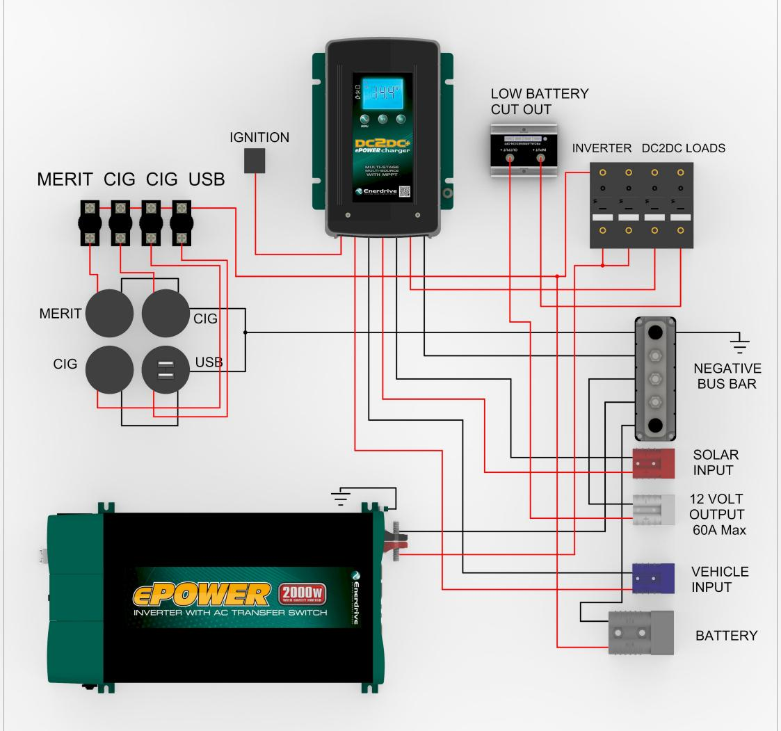
This wiring diagram is only a representation on how the wiring is done and may not fully reflect exactly how your system is wired.
