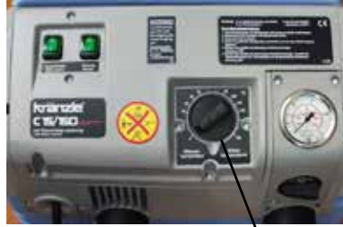
Thermostat with rotary control switch
