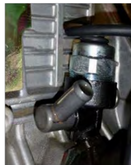
Injector pump inlet
