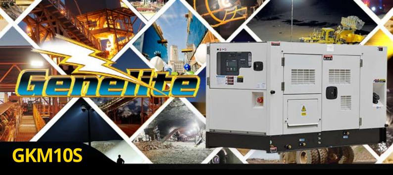
Model GKM10S Type Medium Duty Speed 1500 RPM Phase/Voltage 3, 415 Frequency 50 Hz Stdby Power 11kVA / 9.0kW Prime Output 10kVA / 8.0kW Noise Level (dBA @ 7m) 59dB(A) Fuel Capacity 33 Litres Length 1.5m Width 0.68m Height 1.081m Weight 528 kg
