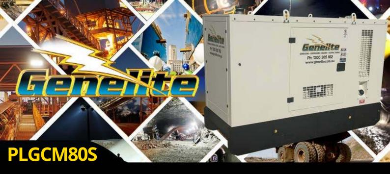
Model PLGCM80S Speed 1500 RPM Phase/Voltage 3, 415 Frequency 50 Hz Stdby Power 88kVA / 70 kW Prime Output 80kVA / 64 kW Noise Level @ 7m 73 dB(A) Fuel Capacity 450 Litres Length 2.86m Width 1.11m Height 1.965m Weight 2035 kg
