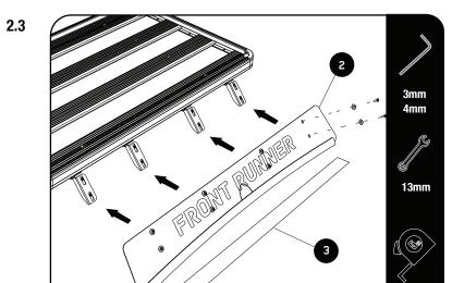
Remove the M5x16 Countersink Screws & M5 Finishing Washers from the bracket.
