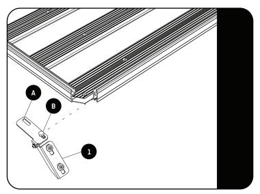
Slide 4 loosely assembled Wind Fairing Adjustable Brackets (Item 1) into the bottom T Slot as shown. Use either Slot A or B as shown in Figure 2.2.
