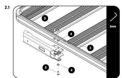
Slide two M8 Nyloc Nuts (Item 3) into the top of the side profile, using to open at the back of the corner.
