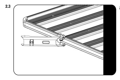
To open the Tap Extension Bracket, pull the knob of the index pin.
