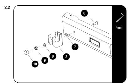
Secure the Shower Holder (Item 2) to the Tap Extension Bracket using a M6 x 16 Button Head Bolt, M6 Nylon Washer, M6 x 12 x 1SS Flat Washer and M6 Nyloc Nut (Items 6, 7, 8 & 9) as shown.
