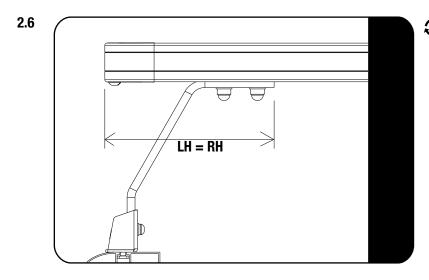
Center the rack on the Legs before fully tightening (LH = RH).
