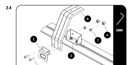
Assemble the Legs (Item 8) to the Leg Mount (Item 3) by using M8 x 30 Button Heads and M8 nyloc Nuts (Items 4 & 7) and the M8 x 20 T-Bolts (Items 1).
