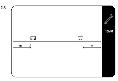
Looking from the side of the vehicle, position the Leg Mounts (Item 3) to center the Slimline II Rack or place Load Bars where desired over the load bed.
