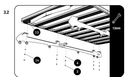
Fit your Roof Rack to the Foot Rails using M8 x 20 Hex Bolts, M8 x 16 x 1.6SS Flat Washers and M8 Nyloc Nuts (Items 6, 13 & 14).
