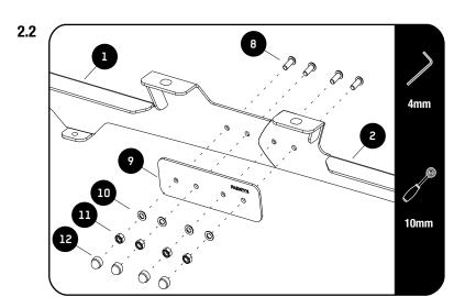
Assemble the front and rear Foot Rail (Items 1 and 2) with the Joiner Plate (Item 9) using M6 x 16 Button Head Bolts, M6 x 10 x 1SS Flat Washers and M6 Nyloc Nuts (Items 8, 9, 17 & 10) as shown.
