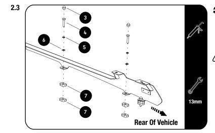
Place a bead of silicon around each of the M8 x 40 Hex Bolt threads.
