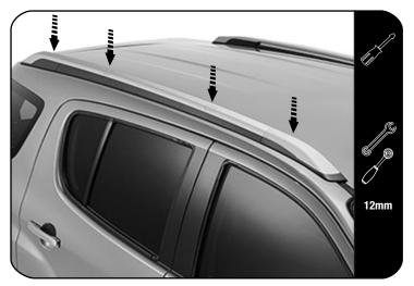
Before you start with the fitment of the Foot Rails (Items 1 & 2), you need to remove the factory roof rails.
