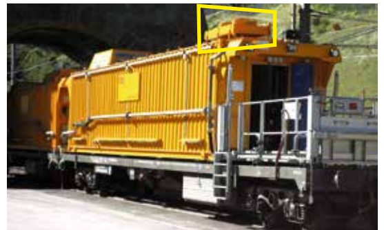
Radiator mounted separately on wagon roof
