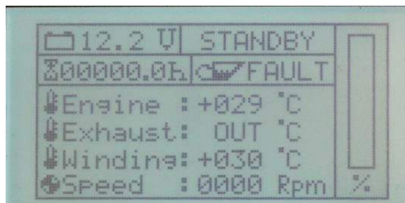
Fig. 6.2-1: Fault: „Cylinder head temperature out of range“
