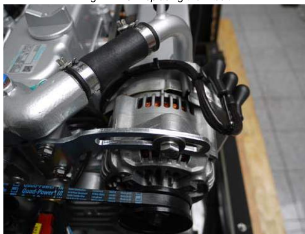
Fig. 1.21-4: Replacing the V-belt
