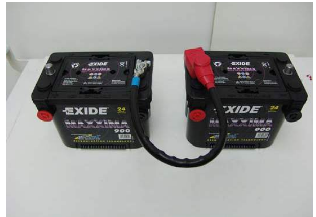
Fig. 5.6.2-3: Installation starter battery
