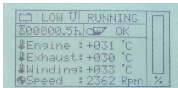
Fig. 14.1.1-1: Warning: „Battery power too low“
