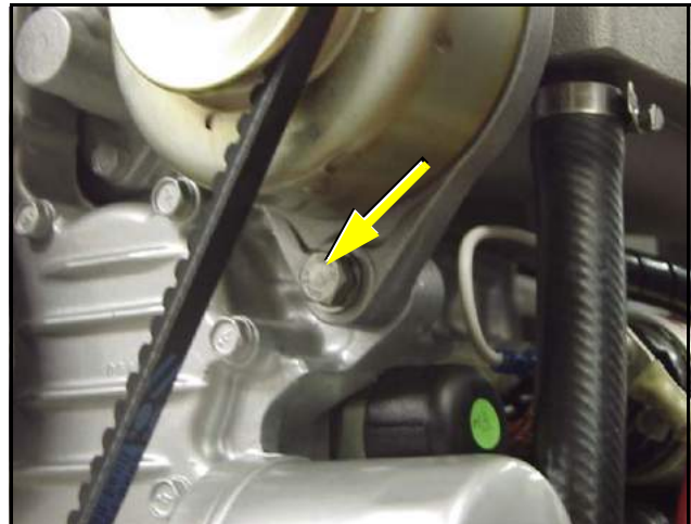
Fig. 7.11-2: Screw underneath the alternator
