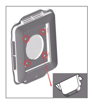
• Fix the plenum assembly on the plenum mounting
