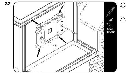
Decide where you would like to mount the bracket assembly and mark the center of the 4 slots indicated in fig 2.2.
