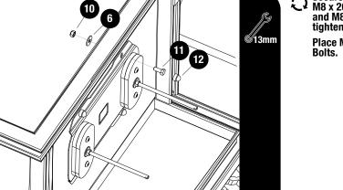
C) Secure the Bracket to the trailer using M8 x 20 Hex Bolts, M8 x 25 x 2 Flat Washers and M8 Nyloc Nuts (Items 6, 10 & 11). Fully tighten.
