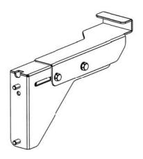
( **B** ) Using Step 2A as a guide, loosely assemble the Corner Wings (Items 23, 24, 25) as shown.
