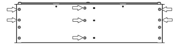
( F ) Using six M6 x 20 Hex Hex Bolts, six M6 Spring Washers and six M6 x 19 Flat Washers removed in Step 2E, secure the Rear Support (Item 22) to the back of the Drawer System as shown.
