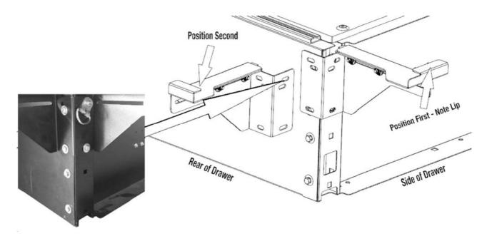
( **D** ) Secure the front and rear of the Drawer System to the vehicle using the 37 mm C-hooks and Turnbuckles (Items 2 & 35) as shown below. Ensure Drawer remains centered, left to right, and 50 mm in from the edge of the load bay (Refer to Step 3A).
