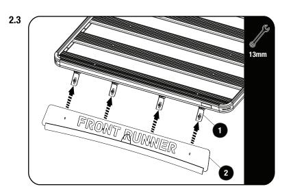
Center the Wind Fairing (Item 2) and position the Wind Fairing Brackets (Item 1) aligning the slotted holes. Fully tighten the Brackets to the rack.
