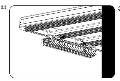
Fully tighten the M8 Nyloc Nuts fitted in 2.1.
