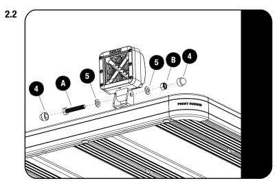
Fit the LED light to the bracket as shown, using the M8 x 45 SS Hex Bolt and M8 SS Nyloc Nut supplied with the light, together with the M8 x 16 x 1.6 Flat Washer and M8 Nut Caps supplied with the Mounting Bracket.
