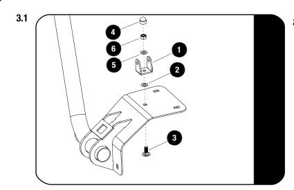
Fit the Mounting Bracket (Item 1) using a M8 x 20 Carrige Bolt, M8 x 16 x 1.6SS Flat Washer, M8 Nylon Washer and M8 Nut Cap (Items 2, 3, 4, 5 & 6) as shown.
