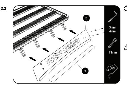
Remove the M5x16 Countersink Screws & M5 Finishing Washers from the bracket.
