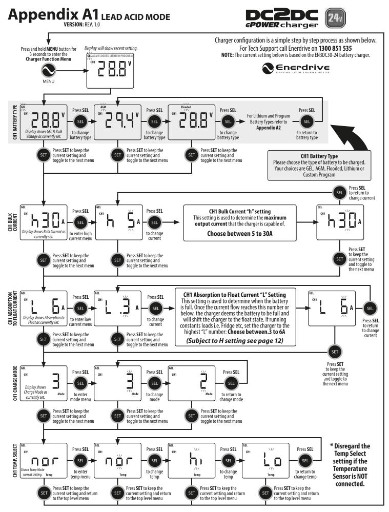
NOTE: At any function setting, pressing the MENU button will exit the function mode.
