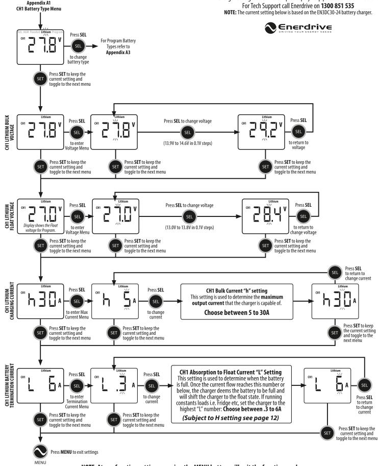
NOTE: At any function setting, pressing the MENU button will exit the function mode.
