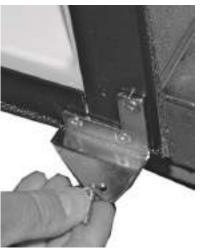
6. Unscrew the three screws and remove lower hinge. Save the screws.
