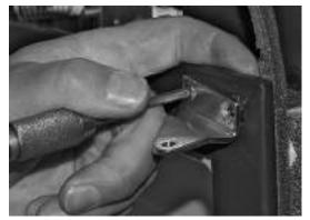
11. Remove the travel catch by unscrewing the two screws. (Save screws and catch.)
