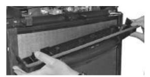
2. Use a socket wrench to loosen the upper hinge pin. Remove pin and save for later use.
