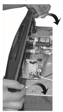
Remove the panel and place it on soft material to avoid scratches or marks.
