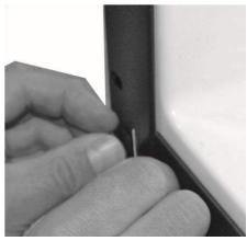
8. Locate the new hinge. Insert hinge pin into hinge hole. Secure the hinge with the three screws removed earlier.
