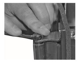
3. Lift the door off the lower hinge pin.
