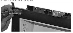
Locate the door. Unscrew screws and remove lock plate and plug. Replace in opposite positions.
