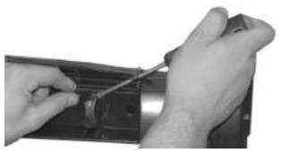
If the top part of the refrigerator is accessible, you can remove the knobs like this:
