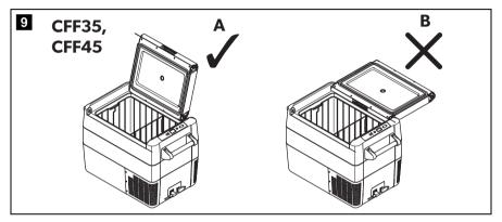
The lid has a built-in stop position (A). Do not force the lid past the built-in stop (B).
