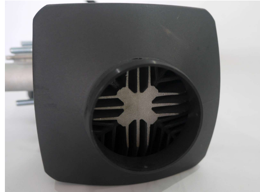
Outlet (hot end)
