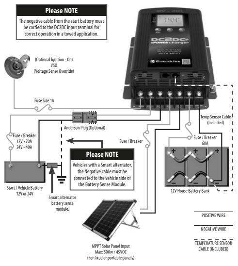
This diagram is for a reference only. No cables, fuse/breakers, batteries or solar panels are supplied with this unit. Local rules and regulations should be followed when installing this unit.
