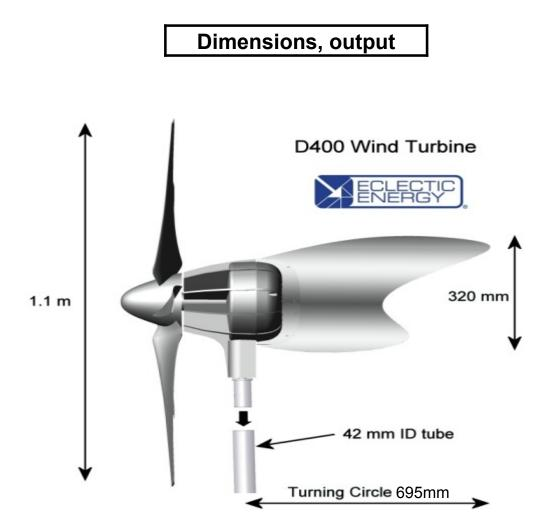
Rated outputs 225 watts at 11 m/s, 400 watts at 16.5 m/s
