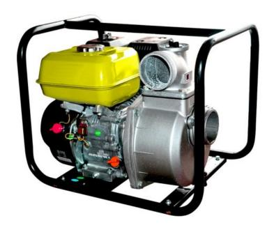
This 3 inch petrol pump is for transferring water for dams, water tanks. The pump outputs 900L/min water at a total head of 30m. It comes with a 2 inch reducer attachment allowing to use 2" hoses on your pump. Note: Using a 2" reducer will reduce maximum pump performance.
