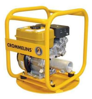
This 6.0hp Drive Unit will drive 2 (50mm) Submersible Flexible Drive Pumps such as Crommelins FP2T model and and Concrete Vibrators.
