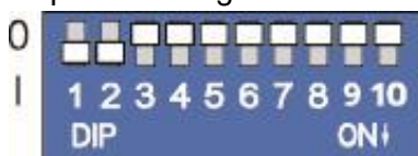
Figure 4: DIP switches (factory settings)
