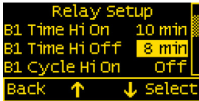
Relay Setup Screen with Relay Normally = On (Closed)
