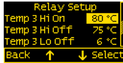
Relay Setup Screen with Relay Normally = Off (Open)
