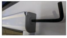
This will unscrew the larger plug and will be already putting more tension on the spring. Usually 3 to 6 turns should add sufficient tension. When enough tension is achieved, while still holding plug against container let it turn clockwise a little and the plug will lock itself back in.
