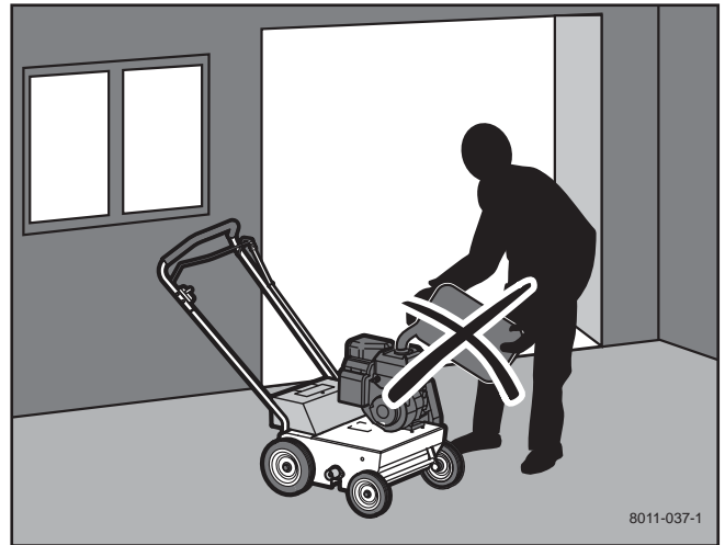
Never fill the fuel tank indoors.
