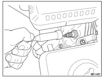
Remove the spark plug cable.
