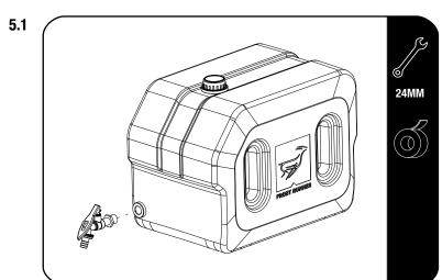
When fitting the tap, apply thread tape to the thread of the tap.
