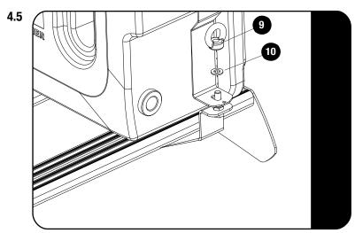
Sure the front of the Strap to the M8 x 30 Hex Bolt inserted in 4.1 using a M8 Eye Nut and M8 Nylon Washer (Items 9 & 10) as shown.
