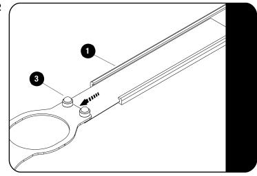
Ensure that the one end of the Strap Rubber (Item 1) is moved up against the end of the Rear Strap (Item 3).
