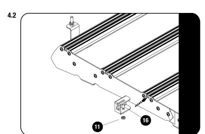
Assemble the M8 x 16 Button Head and M8 Thin Nut (Items 11 & 16) to the Rear Mount Bracket (Item 5).
