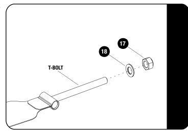
Loosely fit the M6 Nyloc Nut and M6 x 12 x 1 Flat Washer (Items 17 & 18) to the T-Bolts at the ean for the Rear Strap as shown.
