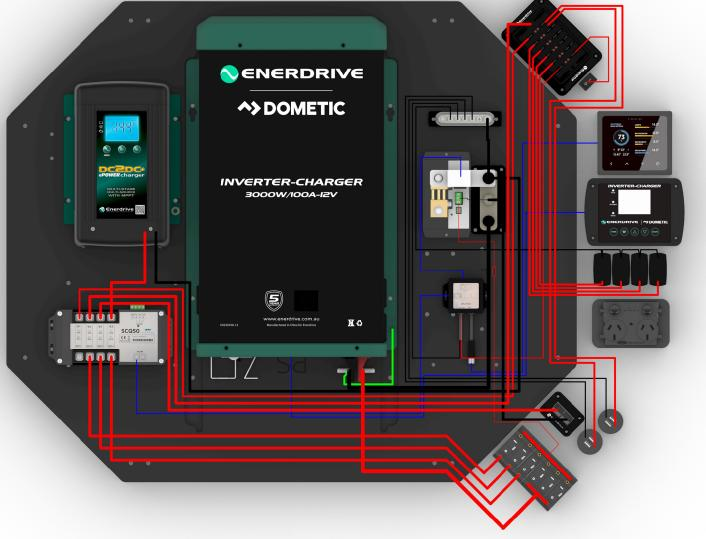
NOTES: CABLE SIZES: PROJECT: VOYAGER ALL EXTERNAL CABLE SIZES 95mm2 1mm2 DRAWING NAME: DRIVER WIRING DIAGRAM PROVIDED ARE A GUIDE ONLY. **ENERDRIVE** Pico Cable LOAD REQUIREMENTS MAY VARY, PLEASE SIZE ACCORDINGLY. DRAWN BY: DATE: 27/07/23 M. MCDOUGALL Comms Cable IF UNSURE, REFER TO LOCAL (as required) DATE: 27/07/23 APPROVED BY: D. BALL STANDARD REGARDING CABLE SIZING FOR EXTERNAL LOADS. 4mm2 SCALE: SHEET: 1 OF 1 1:5.5
