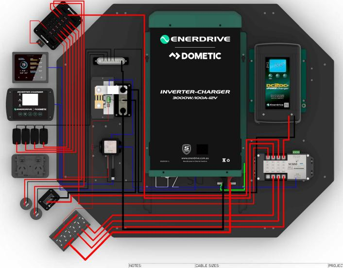
PROJECT: **VOYAGER** ALL EXTERNAL CABLE SIZES = 1mm2 DRAWING NAME PASSENGER WIRING DIAGRAM 95mm2 PROVIDED ARE A GUIDE ONLY ENERDRIVE Pico Cable LOAD REQUIREMENTS MAY VARY, PLEASE SIZE ACCORDINGLY, DRAWN BY: M. MCDOUGALL Comms Cable IF UNSURE, REFER TO LOCAL (as required) APPROVED BY STANDARD REGARDING CABLE D. BALL SIZING FOR EXTERNAL LOADS. = 1.5mm2 4mm2 SCALE: 1:5.5
