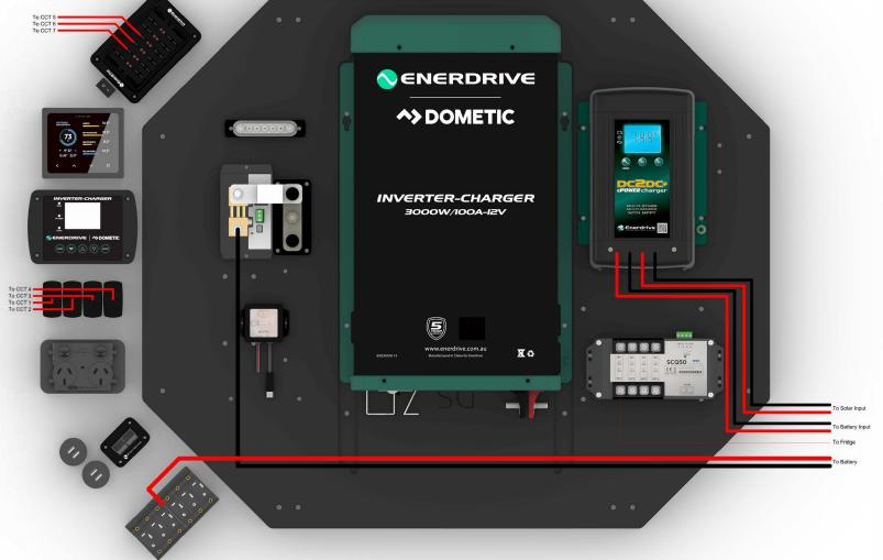
NOTES: CABLE SIZES: PROJECT **VOYAGER** ALL EXTERNAL CABLE SIZES = 1mm2 95mm2 PASSENGER WIRING DIAGRAM PROVIDED ARE A GUIDE ONLY INSTALLER Pico Cable LOAD REQUIREMENTS MAY VARY, PLEASE SIZE ACCORDINGLY DRAWN BY: DATE: 27/07/23 M. MCDOUGALL Comms Cable IF UNSURE, REFER TO LOCAL (as required) DATE: 27/07/23 APPROVED BY STANDARD REGARDING CABLE D. BALL SIZING FOR EXTERNAL LOADS. = 1.5mm2 4mm2 SCALE: SHEET 1 OF 1 1:5.5
