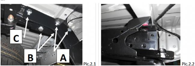
2.1 Lift towbar between the chassis rails and insert fasteners **A** as shown on Pic.2.1 and Scheme 1 and finger tighten fasteners
