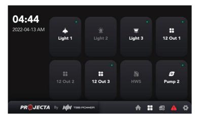
The load control page displays all switchable outputs with their functions named. When the load is turned on, the load icon is white with a green dot in the upper right corner. If the load is turned off, the icon turns gray and the green dot disappears.
