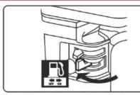
Turn choke lever anf fuel valve lever OFF
