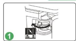
Choke position: START to start cold engine, RUN to restart warm engine
