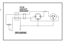
Ground the generator by tightening the grounding nut on the front control panel against a grounding wire. A generally acceptable grounding wire is a **4mm²** (**Australian stranded copper wire**).
