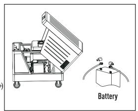
3. Remove the cover from the battery's negative (-) terminal and connect the black cable to the battery's negative (-) terminal.
