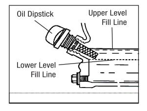
For subsequent operation, the oil level should be checked before each use, or after every 8 hours of operation. The generator is equipped with a low-oil sensor and will NOT start without a sufficient amount of oil.
