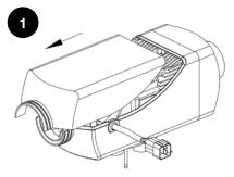
After removal of the outer metal cover of the heater, you can access the heater unit. Replacement of the glow plug can be done without removing the heater unit from the case, however you might find it easier to remove it if doing additional work.
