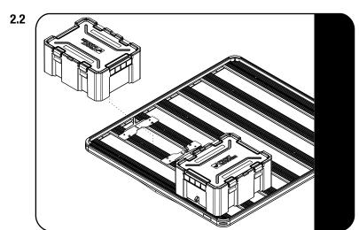
Place your Wolf Pack Pro onto the rack between the Wolf Pack Pro catch brackets. Move the brackets sugly against the Wolf Pack Pro before fully tightening.
